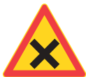
Intersection with equal roads (give way to the vehicles coming from the right)
